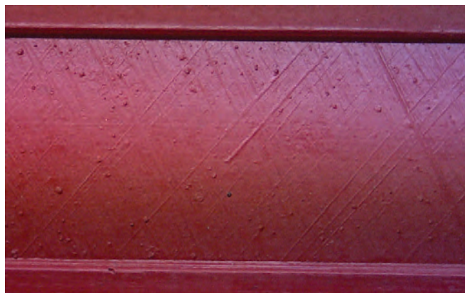
Figure 1: An example of honing marks found in a Colt pistol
