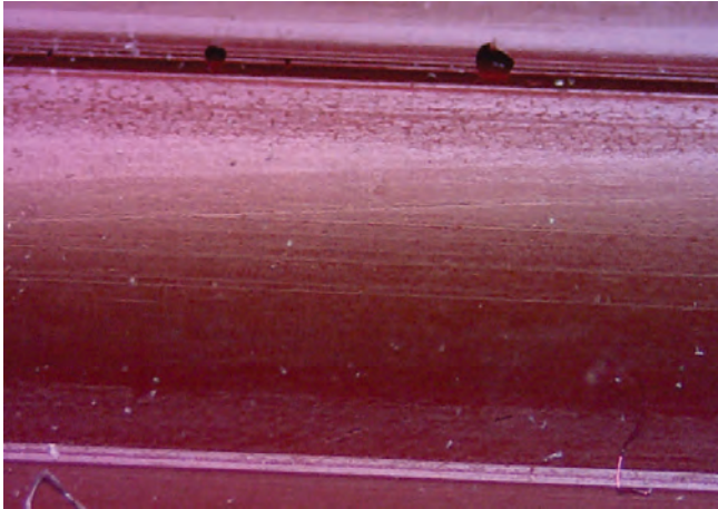
Figure 3: An example of burnishing marks found in a Sig Sauer pistol
