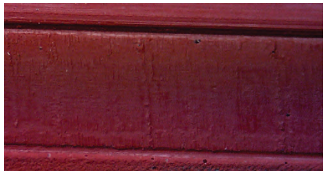
Figure 5: An example of a button rifled land found in a Bryco Arms pistol
