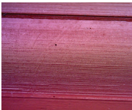
Figure 6: An example of a broached land found in a Beretta pistol
